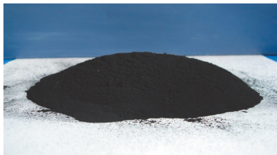
Figure 6 – Pyrolysis carbon black from worn tires
