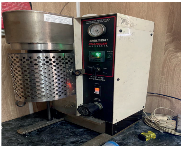
Figure 2 – Chandler Engineering Model 5550 High Pressure High Temperature Viscometer
